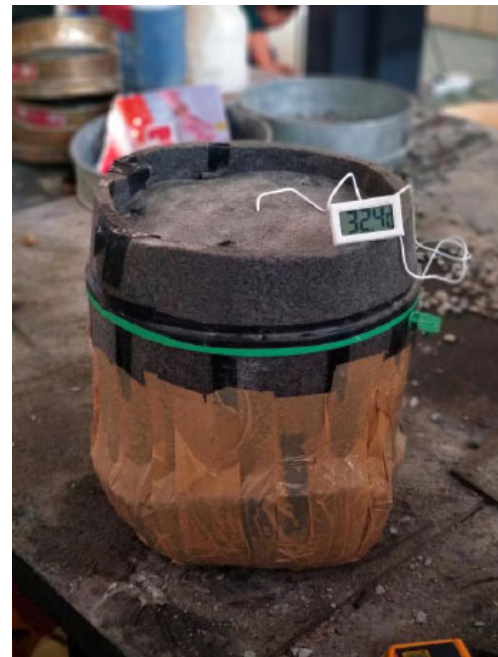
Fig. (4). Experimental arrangements for determination of specific heat capacity.
